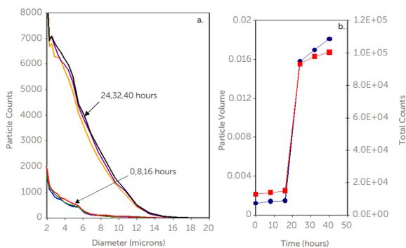
Figure 2. a. PSDs of a silica slurry after being pumped through a recirculation system for 40 hours; b. Graph of percent volume and cumulative particle counts while in recirculation system.
