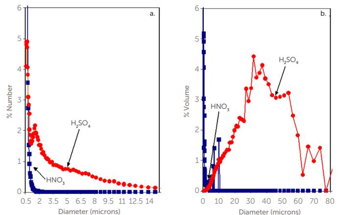
Figure 1. Alumina CMP diluted in sulfuric acid (red, circle) and nitric acid (blue, squares); a. Number weighted PSDs; b. Volume weighted PSDs.
