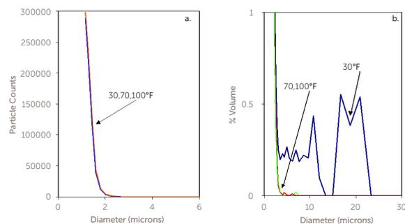
Figure 3. a. Population distributions of cerium oxide slurry at 30, 70, and 100°F. b. Volume weighted PSDs of cerium oxide slurry at 30, 70, and 100°F.
