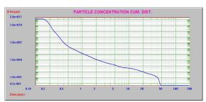
Figure 4. AccuSizer FX Nano silica CMP LPC results.
