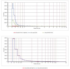
Figure 3. AccuSizer APS silica CMP LPC results.
