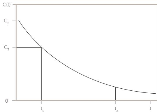
Figure 2. Particle concentration,  $C(t)$ , in the diluted sample suspension that exits the dilution chamber plotted versus time ( $t$ ) for single stage autodilution.
