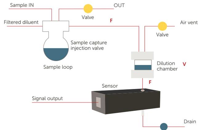
Figure 1. Simplified schematic diagram of a type I autodilution system (single-stage, “continuous-decay” dilution), including an optional sample capture/injection valve.
