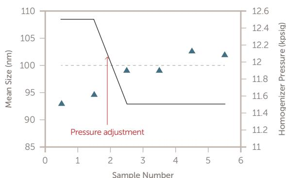
Figure 5. Homogenizer pressure vs. particle size
