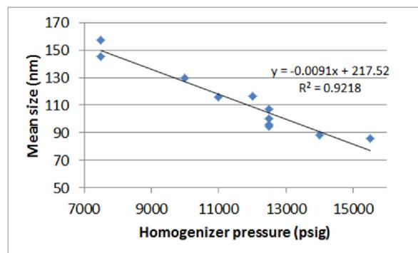
Figure 4. Correlation of pressure to mean size
