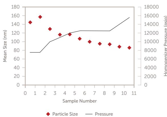
Figure 3. Homogenizer pressure vs. particle size
