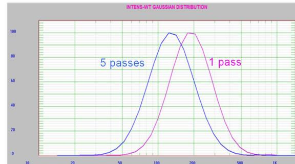
Figure 6. Nanoemulsion sample 329A, 1 and 5 passes, 20k psi.
