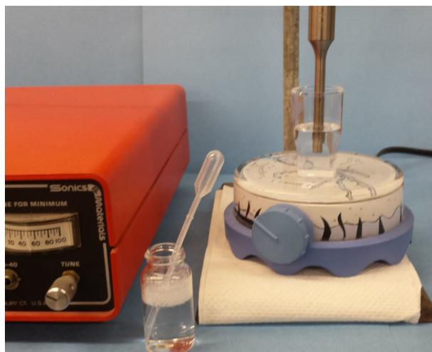
A well organized particle size laboratory should include some of the basic supplies mentioned in this document, such as a range of chemicals, solvents, surfactants, and an ultrasonic probe when dispersing powder.
