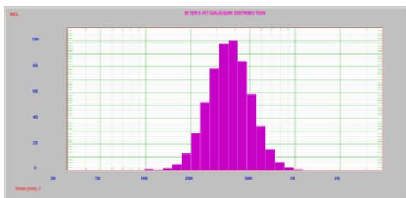
Figure 4. After 30 sec ultrasound, one peak at 385 nm
