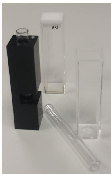
Figure 7. Clockwise starting at the top; 10 mm glass cell, 10 mm disposable plastic cell, round glass cell, round glass cell inside metal cell holder
