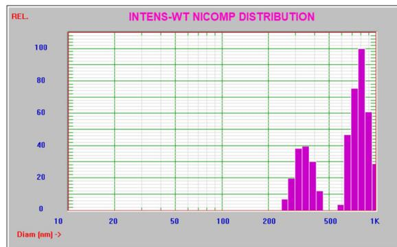
Figure 3. No ultrasound; two peaks at 804 nm and one at 348 nm
