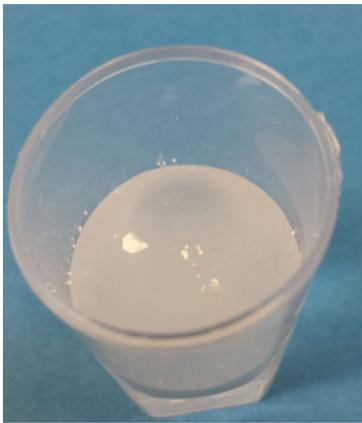
Figure 1. Poor sample powder wetting
