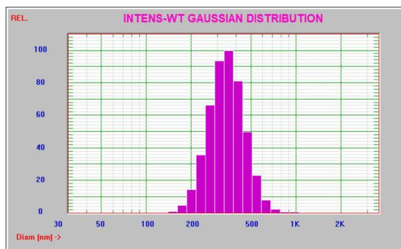
Figure 5. After 60 sec ultrasound, one peak at 355 nm
