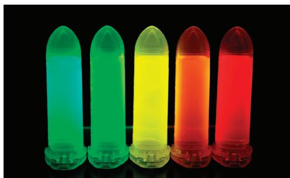
Figure 3. Fluorescent nanoparticles (quantum dots).
