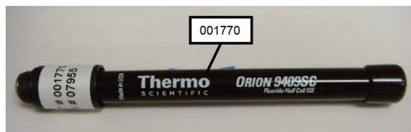
*Fluoride ion selective electrode with protective cap.*
