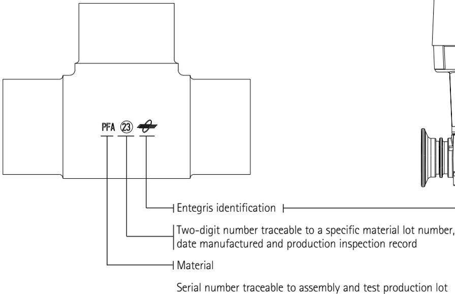
Figure 3: Marking on Valves
