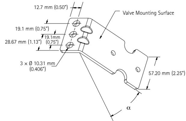
2" orifice valve mounting bracket with 1 1/2" or 2" port connection
