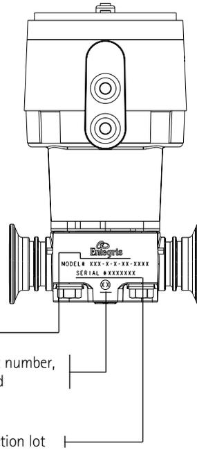
Figure 4: Marking on Saunders® PTFE/EPDM Backed 1" and 2" Diaphragms
