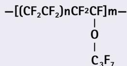
PFA is a fully fluorinated fluorocarbon polymer.
