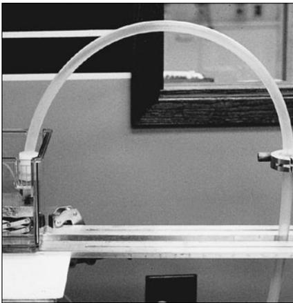
*Determine Leakage Characteristics When Subject to a Side Load*
