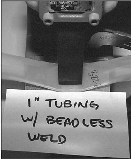
*Weld Strength Test*
