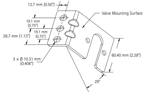
1" orifice valve mounting bracket with 1" port connection
