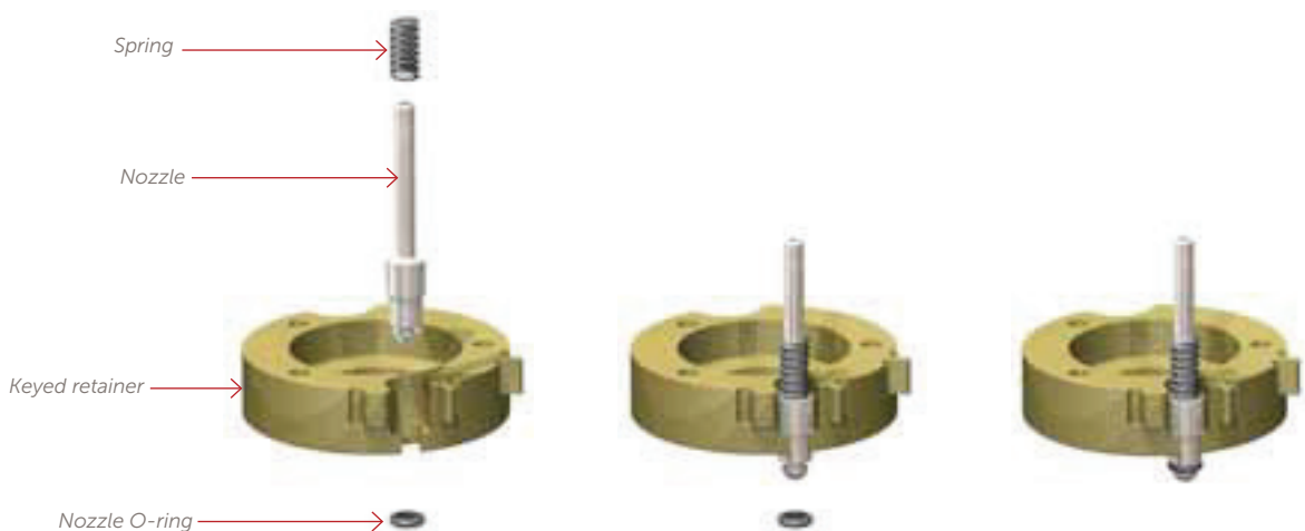
Figure 45. Removing and installing the nozzle, nozzle O-ring and spring.
