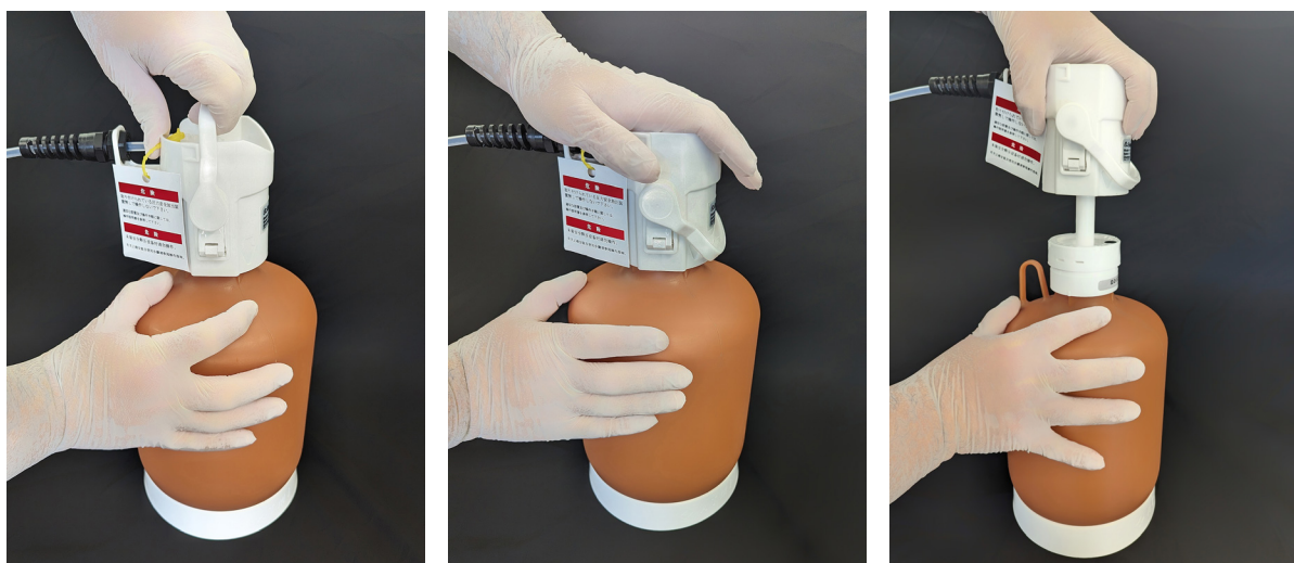
Figure 31. Correct procedure for removing the ErgoNOW connector.
