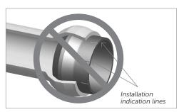
Incorrect installation of insert.
