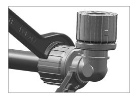
NOTE: Do not overtighten to the point where the nut bottoms out on the fitting body.
