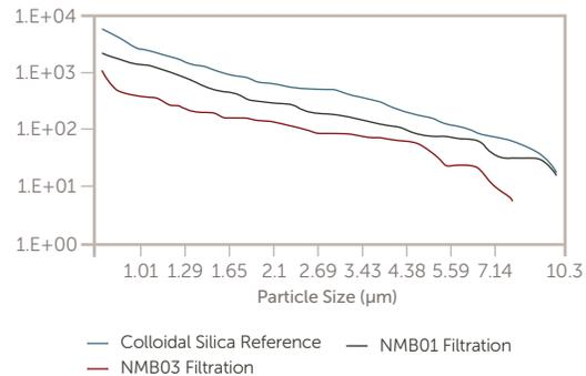
Figure 6. Silica LPC results, NMB01 vs. NMB03
