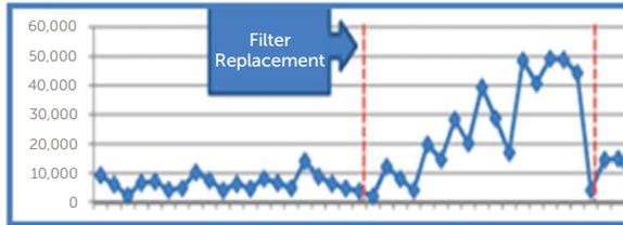
Figure 12. Online LPC downstream of filtration step
