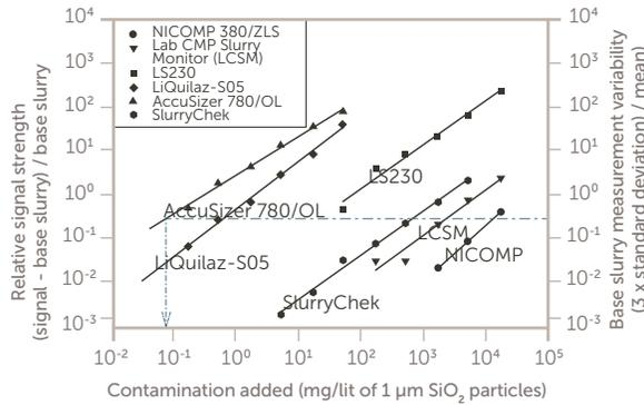
Figure 1. Perturbation detection analysis. From Nichols, K., et. al., *Perturbation Detection Analysis: A method for comparing instruments that can measure the presence of large particles in CMP Slurry*, report published by BOC Edwards, Chaska, MN.
