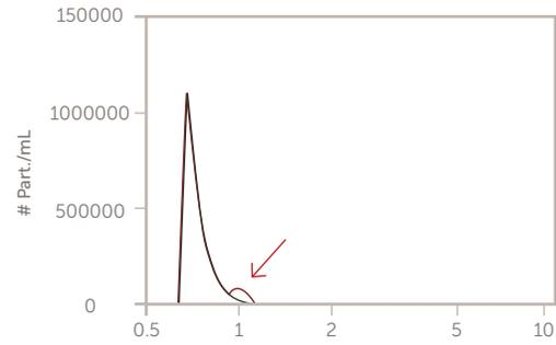
Figure 2. Slurry A before (blue) and after 1  $\mu\text{m}$  spike (red)
