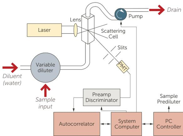
Figure 2. Simplified diagram of DLS system, with autodilution
