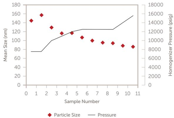
Figure 3. Homogenizer pressure vs. particle size
