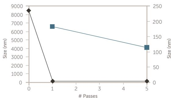
Figure 7. Nanoemulsion sample 329B, unprocessed and 1 and 5 passes, 30k psi.
