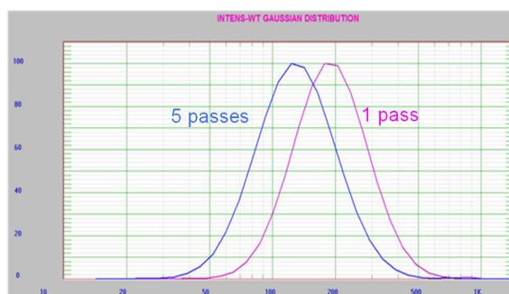
Figure 6. Nanoemulsion sample 329A, 1 and 5 passes, 20k psi.
