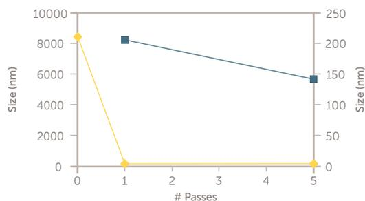
Figure 5. Nanoemulsion sample 329A, unprocessed and 1 and 5 passes, 20k psi.
