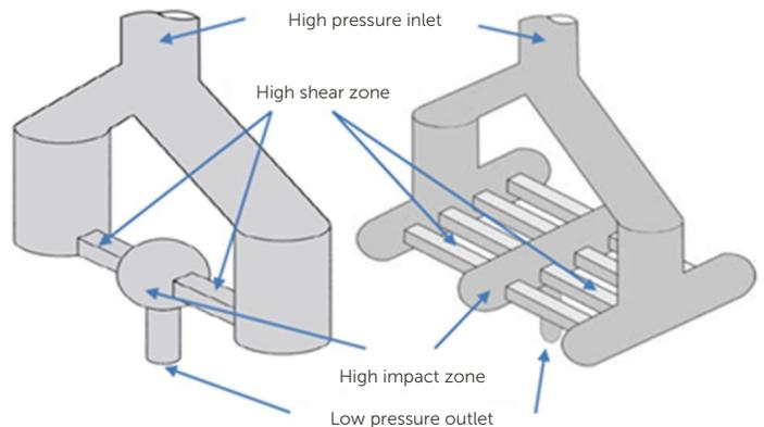
Figure 2. Y single slotted (left) and multi-slotted (right) interaction chambers.
