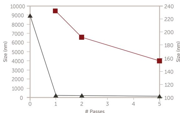
Figure 9. Liposome sample 329C, unprocessed, and processed at 1, 2, and 5 passes, 20k psi.
