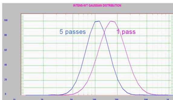
Figure 8. Nanoemulsion sample 329B, 1 and 5 passes, 30k psi.
