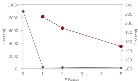
Figure 11. Liposome sample 329D, unprocessed, 1, 2, and 5 passes, 30k psi.
