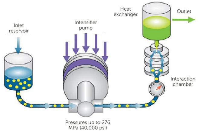
Figure 1. The Microfluidizer process.
