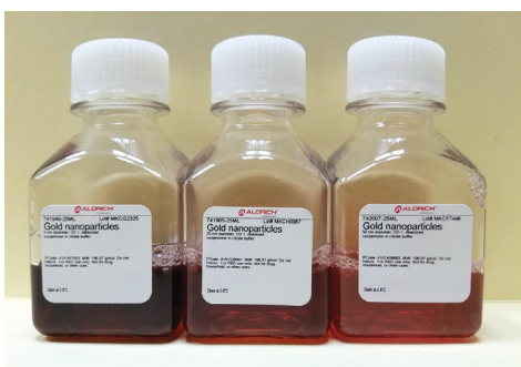
Figure 16. Left to right; 5, 20, and 50 nm Au sample bottles.
