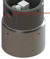
Holes in the upper connector body for the tubing to pass through. These holes prevent the fitting from being turned by the tubing.
