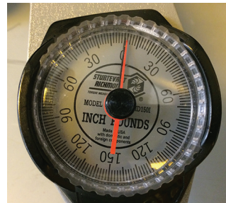
Figure 4. Correctly zeroed torque wrench.
