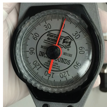
Figure 2. NA-33 0-150 in•lb torque wrench.
