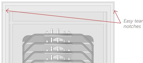
Figure 3. Easy tear notches
