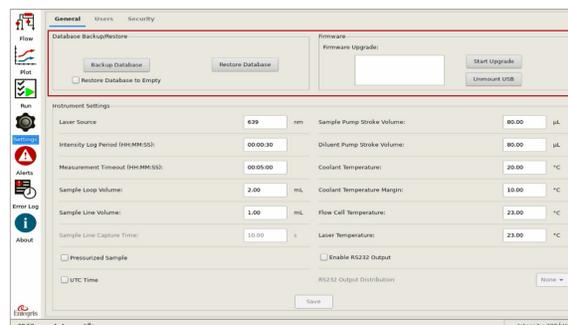
Figure 20. Database backup/restore and firmware upgrade.
