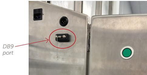
Figure 39. Serial cable connection.
