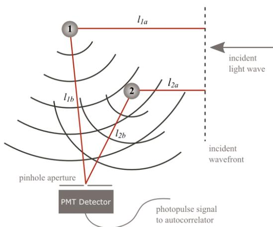
Figure 9. Simplified scattering model (two diffusing particles).
