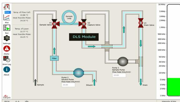
Figure 24. Flow path of a flush.
