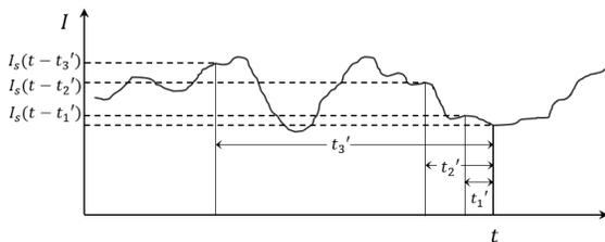
Figure 11. Computation of the autocorrelation function.
