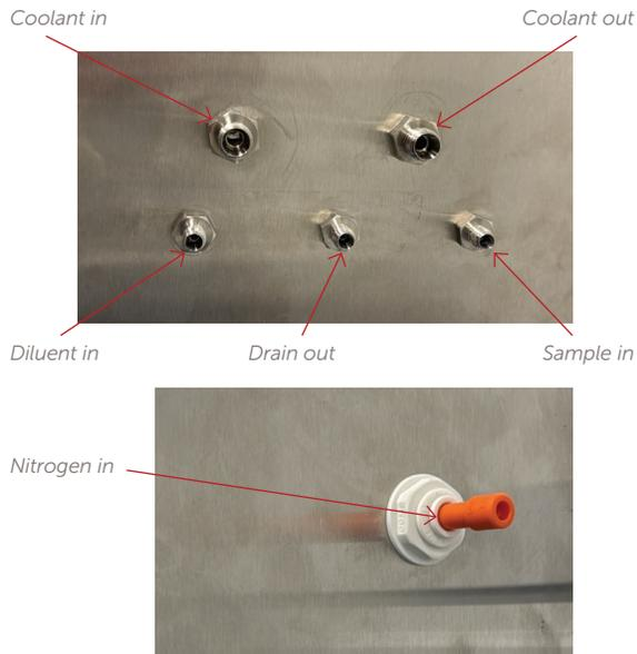
Figure 5. External connections.
