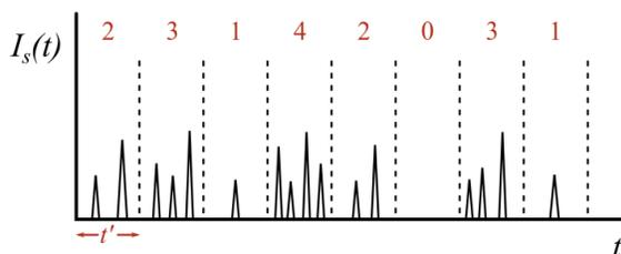
Figure 12. A typical photopulse sequence representing  $I_s(t)$  divided into time intervals of width  $t'$ .
