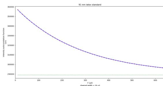
Figure 13. Autocorrelation function for a 91 nm latex standard.
