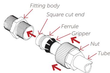
Figure 49. Tubing connections.
