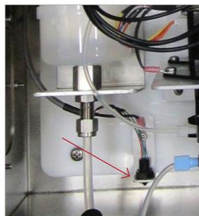
Figure 37. Leak detector.
