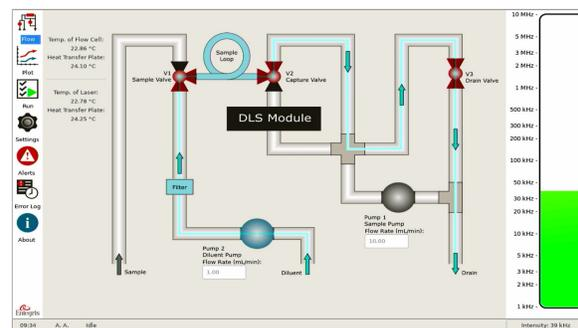
Figure 38. Flow screen operation.
