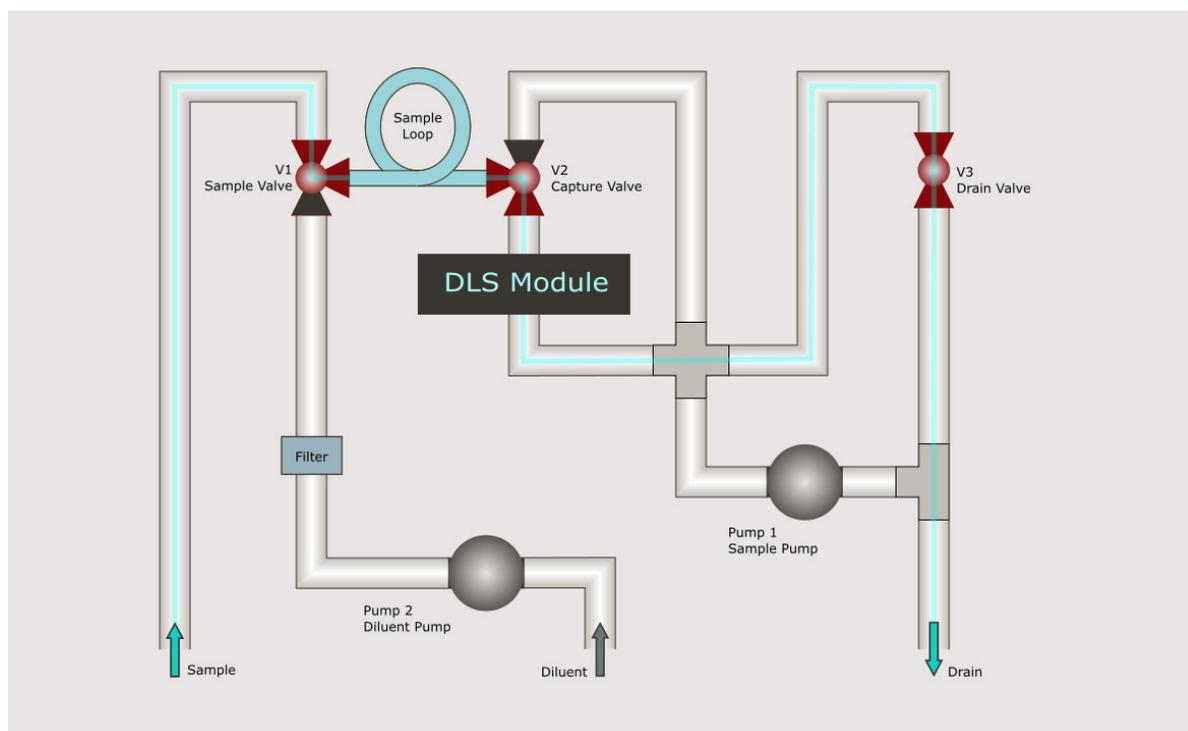
Figure 48. Sample flow cell.
