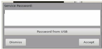
**NOTE: To prepare a USB flash drive for the Password from USB option, copy a service key to a \*.txt file and save this file to the flash drive. Then connect the flash drive to the USB port.**
