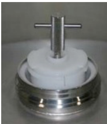
Figure 15. NA-13 diptube removal tool.
