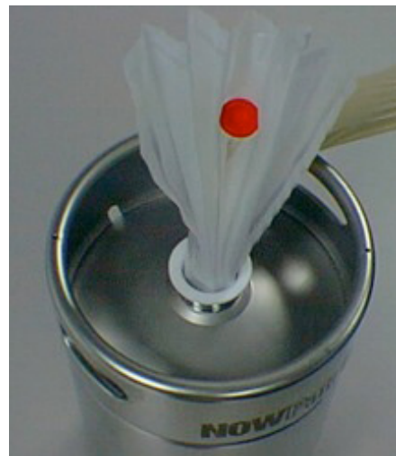
Figure 18. Liner being inserted into canister (observe liner folds).
