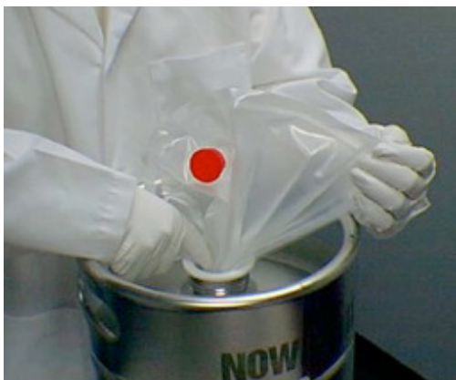
Figure 20. Tucking in the liner layers.
