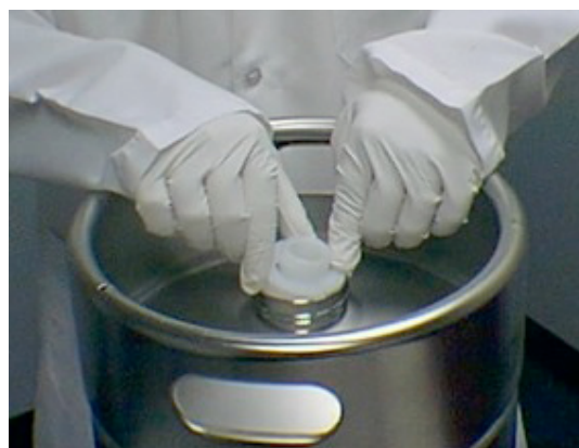
Figure 22. Seating the fitment and retainer into the canister.
