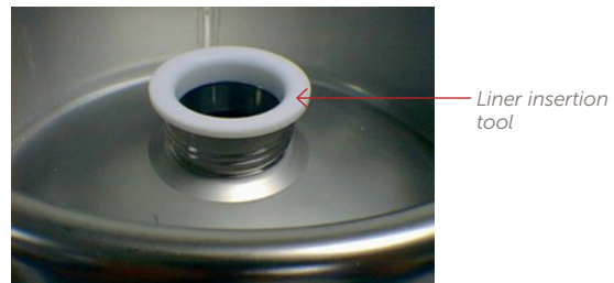
Figure 17. Liner insertion tool inserted in canister neck (NA-60 shown).
