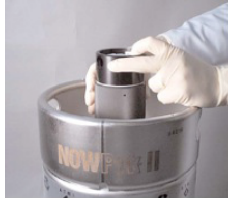
Figure 44. Installing the dispense connector (ND-CD shown).
