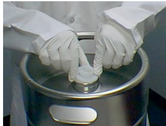
Figure 26. Seating the fitment and retainer into the canister.
