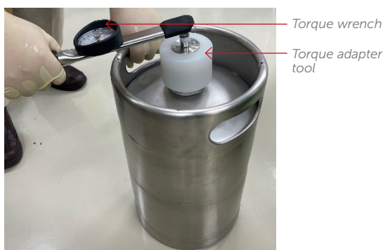
Figure 14. Removing the closure (19-liter canister shown).
