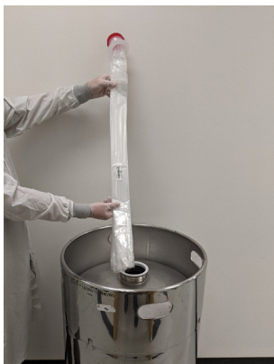
Figure 24. Liner being inserted into canister (observe liner folds).
