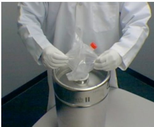
Figure 19. Separating the liner layers.
