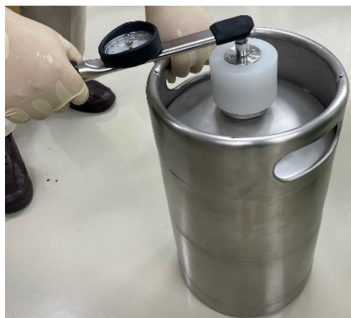
Figure 33. Installing and tightening the two-piece closure.
