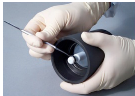
Figure 41. Removing dispense connector O-rings (ND-CD shown).
