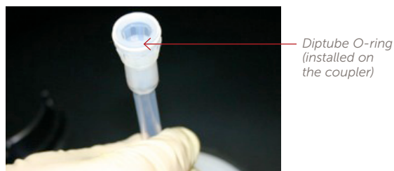
Figure 39. Removing the diptube O-ring.
