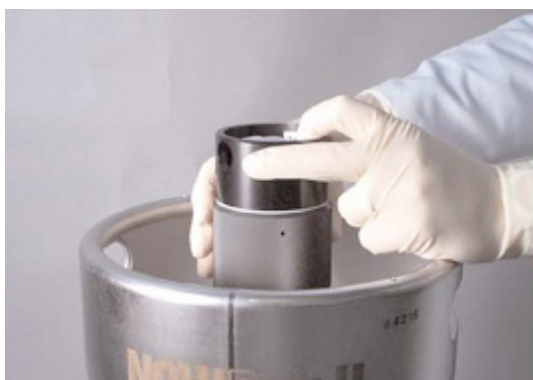
Figure 45. Removing the dispense connector (ND-CD shown).
