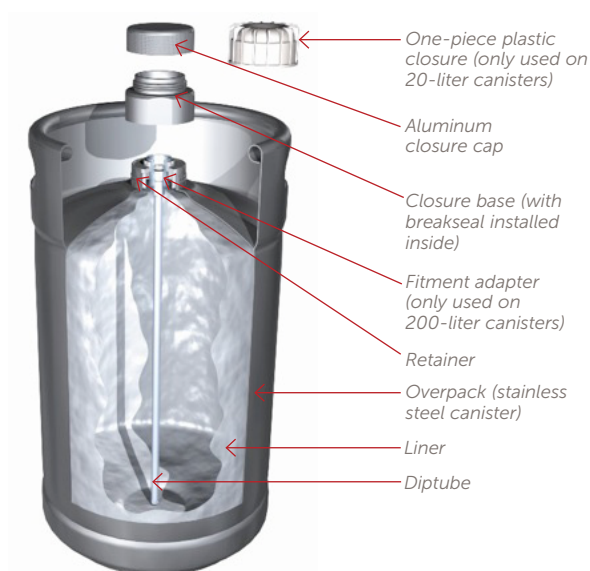
Figure 2. Stainless steel canister with installed components (cutaway view).
