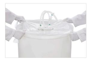
7. At the top of the bag, there is an opaque tubing loop.
