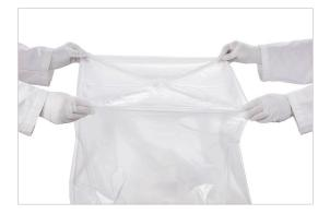
5. The bag should then be inverted, and the top of the bag should be squared using the same method.
