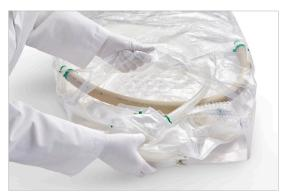
4. The Flex Mixing Bag is designed with BIB (bag-inbag) technology to provide no weld seams on the sides of the chamber. The top and bottom of the assembly should be squared before use. To square the bag, two technicians should locate the bottom of the bag. This can be done by identifying the side with no porting and the stainless steel mixing head (below).
