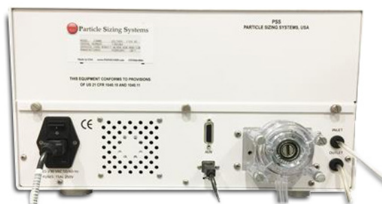
Figure 2. Flow pump and inlet/outlet tubing.
