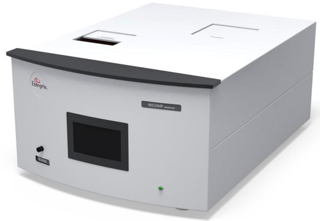
Most dynamic light scattering (DLS) systems have been designed to work at a fixed angle, either 90° or backscatter. No single measurement angle is ideal for every possible sample. For very small particles the scattering is equal at all angles, so any angle is acceptable. But for particles that are greater around 20 nm the scattering angle can affect results. This technical note explains how scattering angle influences results generated.
