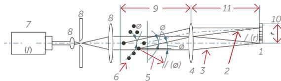
Figure 2. Laser diffraction optics<sup>4</sup>
