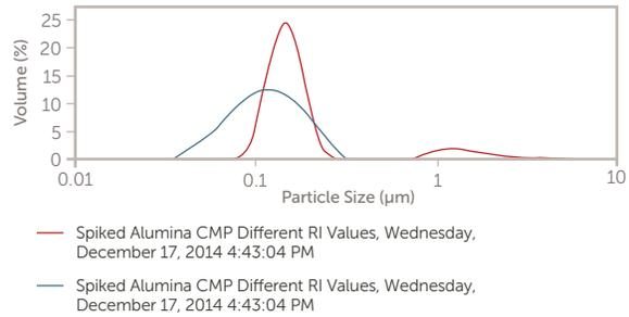
Figure 6. AI CMP slurry spiked with 1 µm PSL
