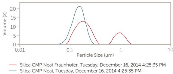
Figure 5. Fraunhofer vs. Mie results
