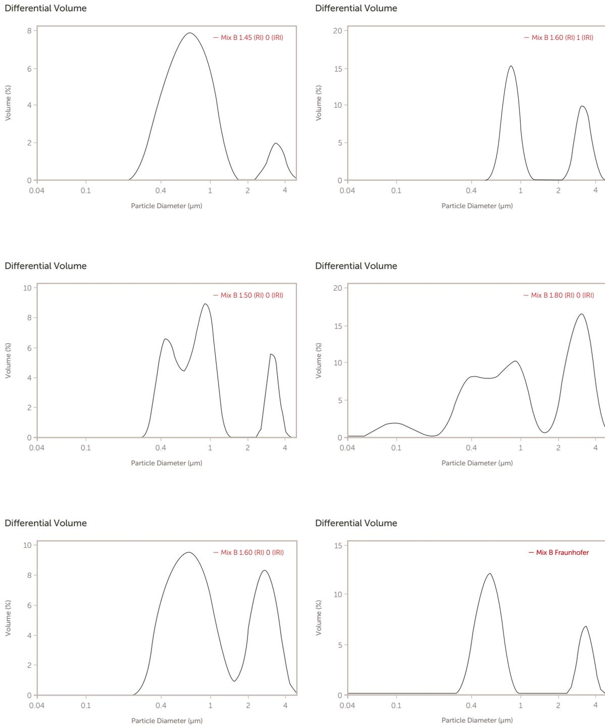
Figure 4. Effect of RI on calculated results
