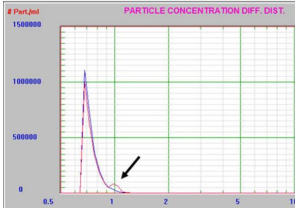
Figure 8. AccuSizer SPOS result of spiked silica CMP slurry
