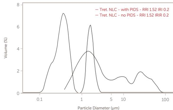
Figure 3. Effect of optics/algorithm
