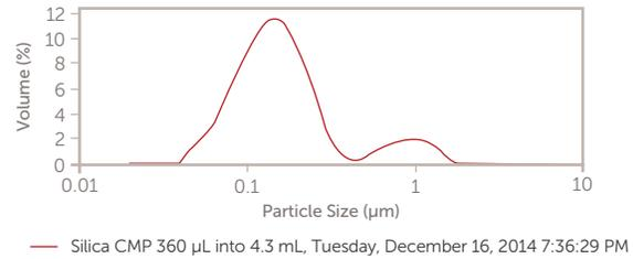
Figure 10. Laser diffraction result; 360  $\mu\text{L}$  into 4.3 mL silica CMP slurry
