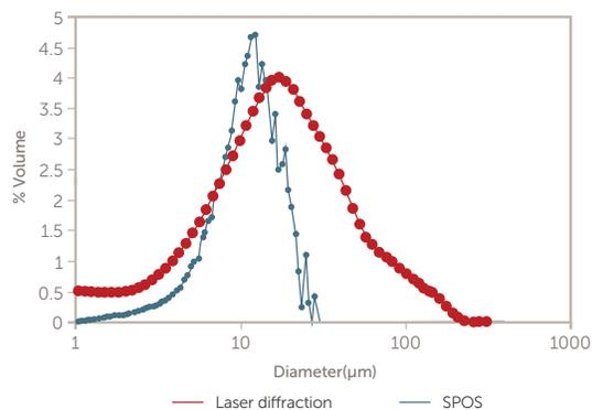
Figure 12. SPOS vs. laser diffraction results for a sieved sample
