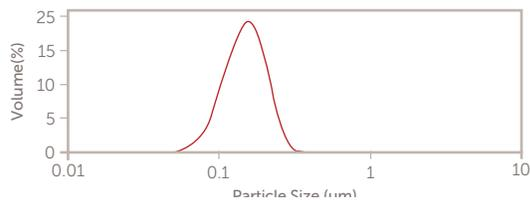
Figure 9. Laser diffraction result, 177  $\mu\text{L}$  PSL into 250 mL silica CMP slurry
