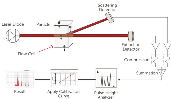
Figure 1. The LE400 SPOS sensor
