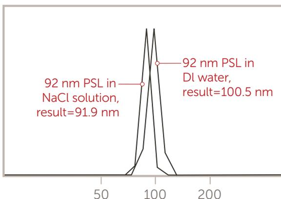
Figure 1. 92 nm PSL results in DI water and 10 mM NaCl Solution
